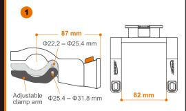
Adjust Clamp Size. Clamp arms have two sets of matching pin holes for smaller or larger diameter handlebars – default position suits most bars. To change setting, push pins out with 3 mm Allen key. Reinsert pin into lower
