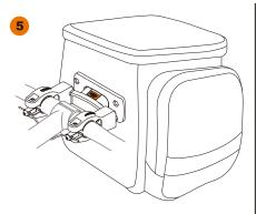
Push bag down, sliding it until it locks into mount. When bag is attached correctly, there should be a distinctive 'click' sound.
