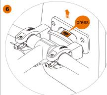
Press button release while pulling bag upwards with strap at rear of bag.
